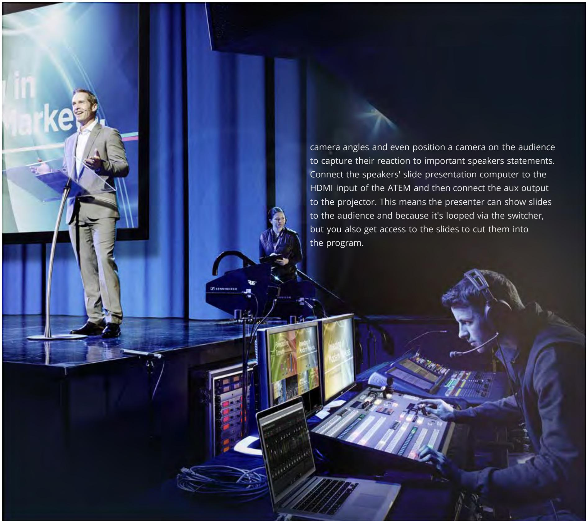
camera angles and even position a camera on the audience to capture their reaction to important speakers statements. Connect the speakers' slide presentation computer to the HDMI input of the ATEM and then connect the aux output to the projector. This means the presenter can show slides to the audience and because it's looped via the switcher, but you also get access to the slides to cut them into the program.
