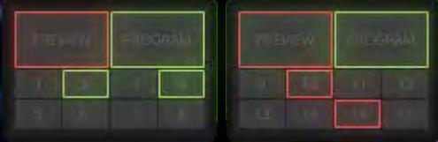
The advanced ATEM 2 M/E Production Studio 4K model features 2 independent multi view outputs so that you can monitor up to 16 cameras simultaneously across 2 screens!
